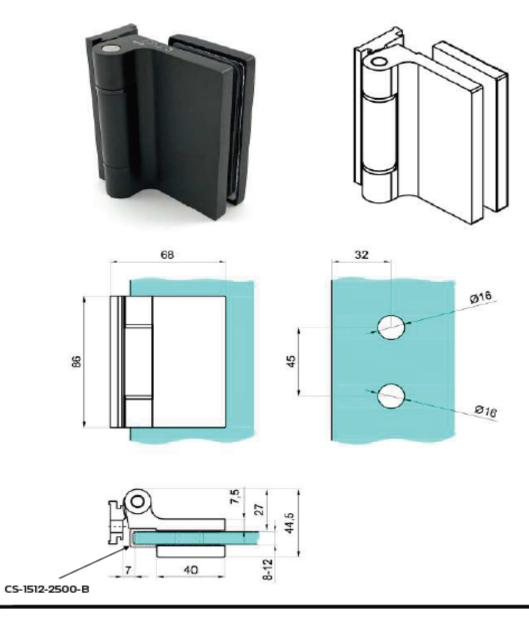
CONNECTION OF CS-1512-2500-B PROFILE WITH NTZ-650-B HINGE DOES NOT REQUIRE PROFILE CUTTING. THE PROFILE IS SLIED ENTIRELY ON THE EDGE OF THE MOUNTED GLASS DOOR.
